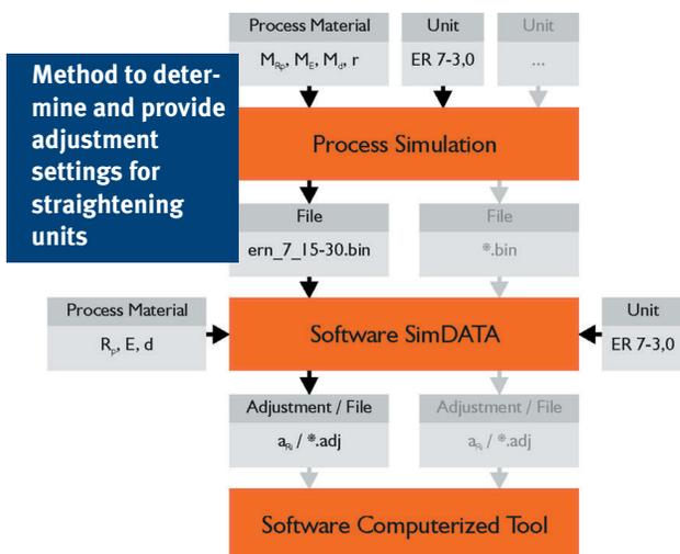
can be moved directly into the wire manufacturing or processing environment. The operators themselves should be given the tools to calculate the required positions of the rolls. To address the complexity of process simulation, a method has been developed based on easy-to-use software, which produces results that allow even an inexperienced operator to determine roll positions, so that a defined level of production quality can be achieved.
