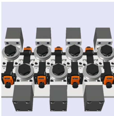
Richtapparat AS 7-20 PO, bestehend aus Richtmodulen AS 1-20 PO.
